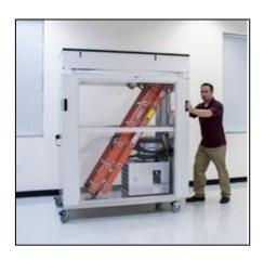
Transport the AG8000 in the fully collapsed position and use the handles located at the corners of the unit to move the mobile containment unit.
