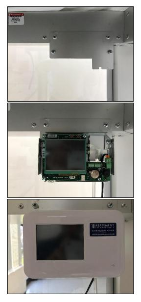
Locate the pressure monitor mounting bracket on the inside back wall of the AG8000.
