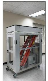
Position the mobile containment unit in the approximate location where ceiling access is required.
