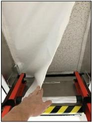
Unzip the zippers on each side and detach the hook and loop on the short side near the ladder to open the top cover.
