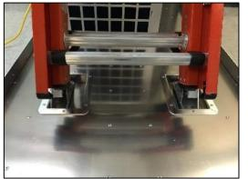
Place the feet of the ladder into the recessed pockets in the floor. Unbuckle the strap on the left side of the ladder that secures the three sections of the ladder together.
