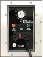
Set the PAS750 to the highest setting on the unit's variable speed control knob.
