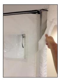
Both the top cover and the fabric enclosure are fastened to the mobile containment unit via hook and loop. To remove the top cover, simply separate the hook and loop along the perimeter of the top cover. To remove the fabric enclosure, detach the hook from the loop from each of the four telescoping members as shown above. Then separate the hook and loop along the top perimeter and then the bottom perimeter.
