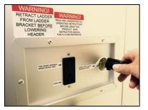
Power must be supplied to the AG8000 in order for any of the outlets to be operational. Plug the female end of an extension cord into the POWER SUPPLY outlet located on the back side of the unit and the male end into a 110V-120V, 60Hz, single phase outlet.
