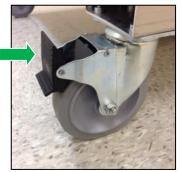
To unlock the casters, push the pedal towards the wheel with work shoe.
