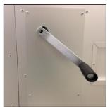
Turn hand crank clockwise to raise the header. Turn hand crank counterclockwise to lower the header.
