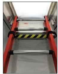
After raising the header to the ceiling, the ladder can be extended and placed against the ladder bracket. Use the hook and loop straps on each side of the ladder bracket to secure the ladder.
