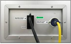
If the PAS750 or PRED750 unit is located external to the AG8000, ensure it is plugged into the outlet labeled "FOR 120VAC VARIABLE SPEED DEVICE ONLY" as shown in the picture above.
