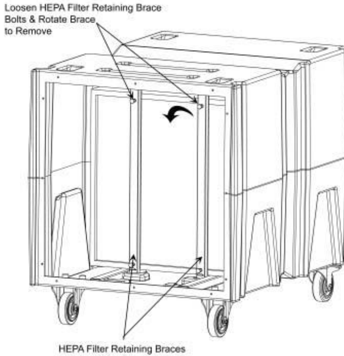
Figure A: HEPA Filter Replacement
